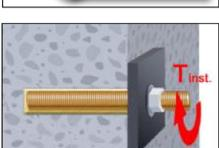
11. After full curing, the add-on part can be installed with up to the max. torque (Table B1 or B3) by using a calibrated torque wrench. It can be optional filled the annular gap between anchor and fixture with mortar. Therefor substitute the washer by the filling washer and connect the mixer reduction nozzle to the tip of the mixer. The annular gap is filled with mortar, when mortar oozes out of the washer.
