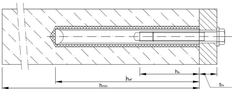
$t_{fix}$  = thickness of fixture
