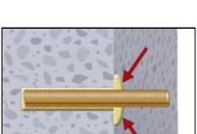
9. Be sure that the anchor is fully seated at the bottom of the hole and that excess mortar is visible at the top of the hole. If these requirements are not maintained, the application has to be renewed. For overhead application the anchor rod shall be fixed (e.g. wedges).
